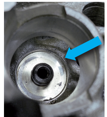
Figure 3: Pressure marks in the cylinder head
