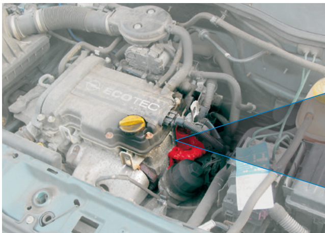
Electric EGR valve in the Opel Corsa (highlighted)
