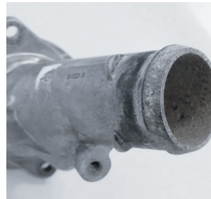
Figure 3: Clean any corroded areas thoroughly prior to assembly.
