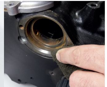
Figure 3: Clean any corroded areas thoroughly prior to assembly.
