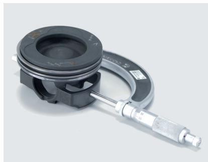
Figure 2: The coating adds approximately 0.03–0.04 mm to the specified diameter
