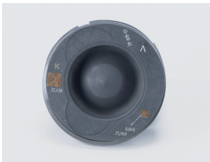
Figure 1: Piston dimensions, fitting clearance, and installation direction are specified on the piston crown
