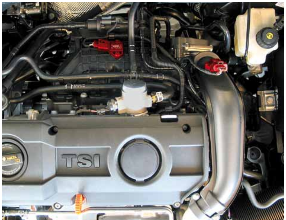
Intake manifold pressure sensor (left) and boost pressure sensor (right) in VW Golf VI (highlighted in red)
