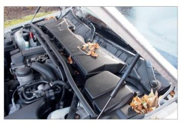
Such faults generally do not constitute a reason for a claim. AIC wiper motors are, same as with OE parts, only **splashproof** and not constructed to be **waterproof**.
