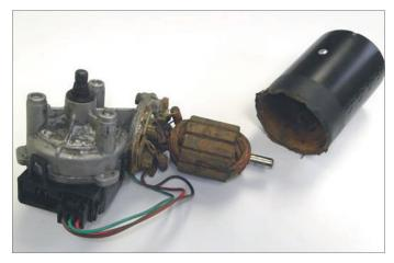
Time and again we receive returns of wiper motors like the one shown in the photo to the left. A quick external glance is enough to already clearly see the rust. The described fault is generally at least sluggish motor performance.
