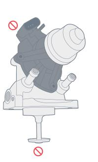
When installing this valve, please be aware, that to avoid damaging the valve, you must connect it to the plug of the car first, while activating your tester function "replace EGR valve" - the valve head will retract slightly, and this will allow you to install it correctly into the cooler module.
