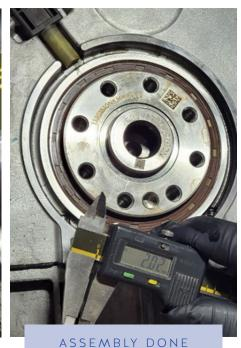
By following these instructions, the rear oil seal 15108100 will be **correctly installed**, optimising leakage protection and engine performance.
