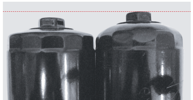
Figure 3: Oil filters, side-by-side comparison—left: normal, right: deformed
