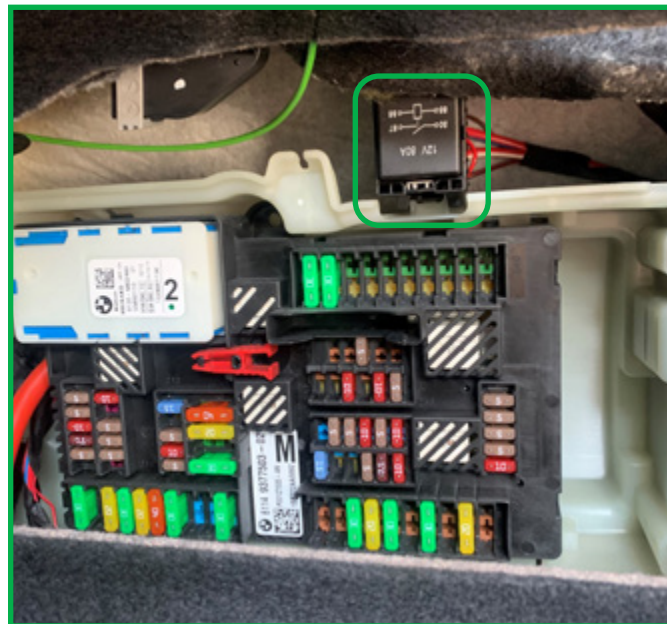
BMW 7 SERIES (F01/02/04) Relay located in the trunk of the vehicle on the right side.
