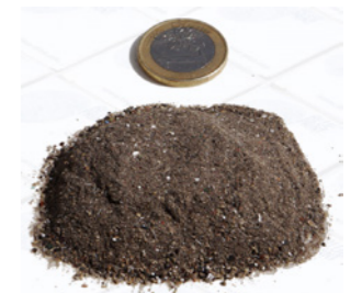
In hard-road conditions, this is the least amount of contamination an air filter will capture during its service life.
