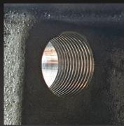
Use an M22 x 1.5mm thread tap to carefully remove any burrs/contamination within the thread of the cylinder head.
