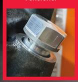
Step 1 Extend the thread within the cylinder head tensioner housing.
