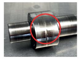
**Damaged camshaft**Causes seizing of the plain
